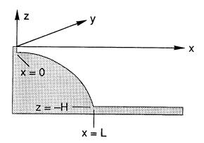
The x axis points offshore while the y axis is alongshore. The shelf-slope region has width L. We start with the shallow water equations over variable topography. We ignore stratification for now and assume that the flow is nondivergent.
